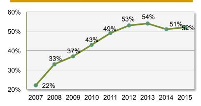
Note: the recovery rates in 2014 and 2015 did not reach high point because leaching time for the new leach pad of Phase II is not long enough.
