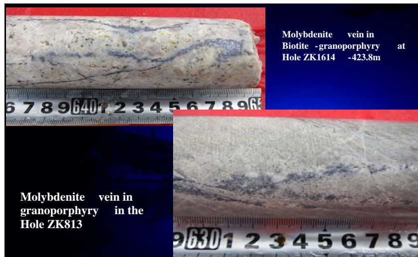
Photo 1, Molybdenite vein in granoporphyry from the core of Hole ZK813 and Hole ZK1614 at Jiama Project
