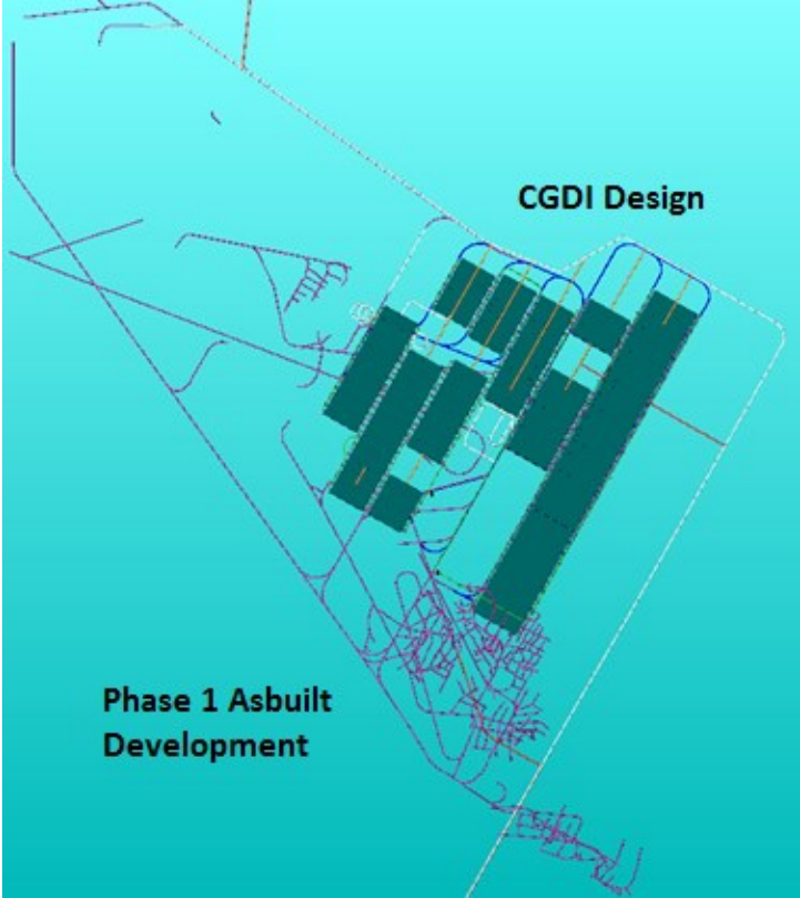
Figure 1-5: CGDI Stopes in Relation to As-built Development
