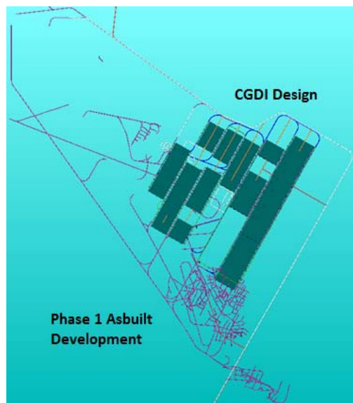
Figure 1-8 CGDI designed stopes in relation to as-built development
